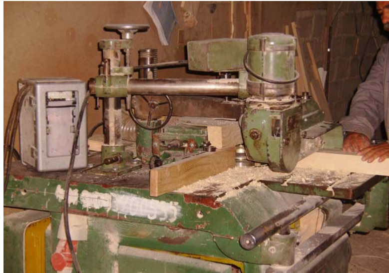
Fig. 2 - Manual milling machine (MNF 10) with automatic
