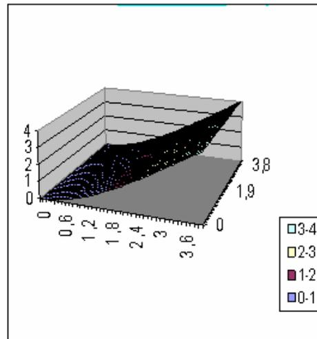
Fig.2 The plate deformation for mode  $i=2, j=1$
