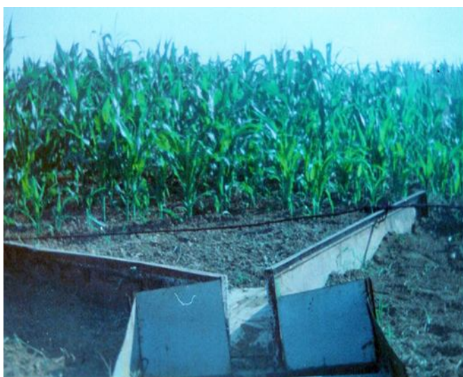
Fig.1 Plots for check flow on the eroded soil from Oradea
