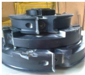
Fig. 3. Set of tools with removable plates for doors and Windows of laminated wood
