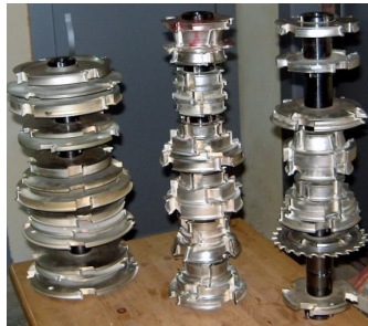
Fig. 3. Set of tools with removable plates for doors and Windows of laminated wood
