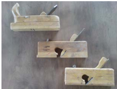
Fig. 4.- Carpenters hand planers.
