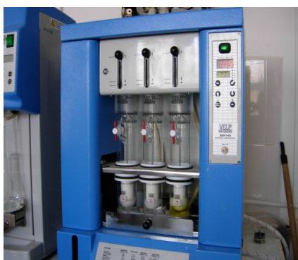
Fig. 1. Soxhlet device for fat assesment
