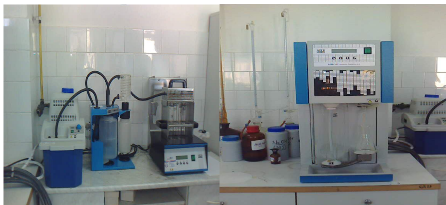
Fig. 2. Protein assessment by Kjeldahl apparatus
