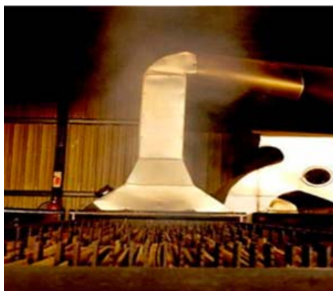
Fig. 9. Oven for heat treatment of staves ( http://pentruvin.ro/index.php?page=butoaie-odyse )
