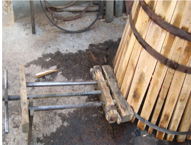
Fig. 7. Tightening bell for the heat treatment of plasticizing
