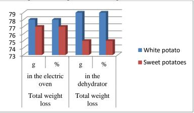
The graphical representation of the total and percentage weight losses of the potato samples used is presented in Fig.3.
