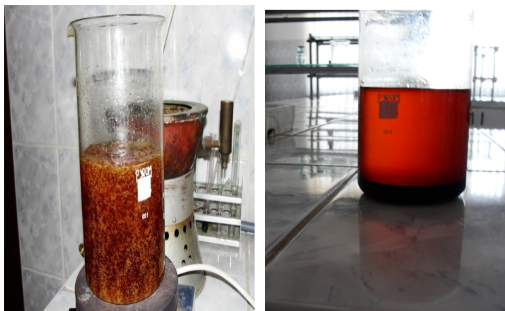
Fig 3. Mixture of biodiesel – glycerine obtained from used palm oil
