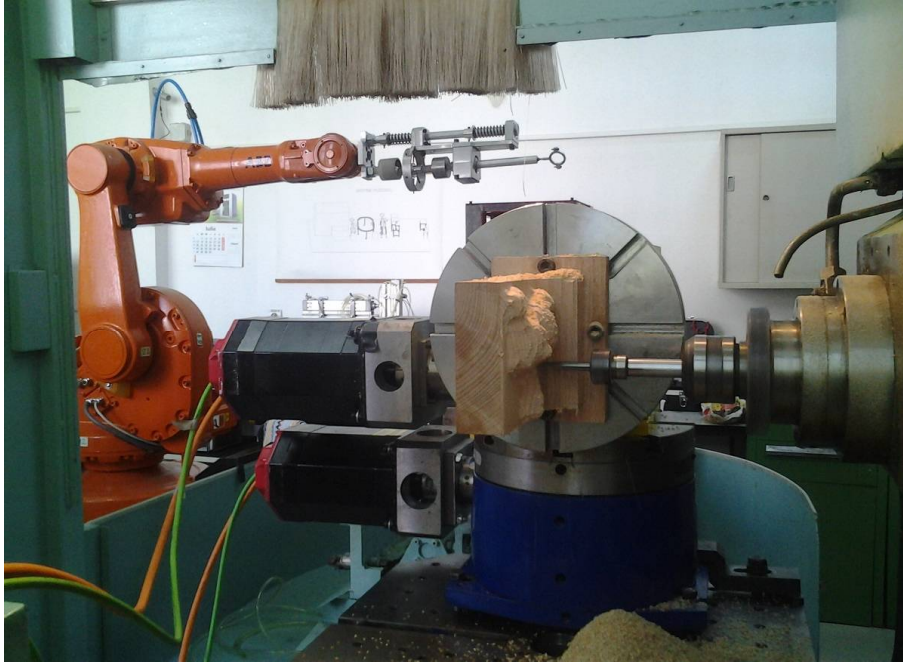
Fig. 5 Sequences during processing (3-axis roughing)
