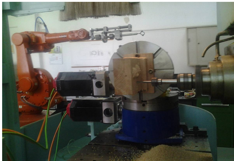
Fig. 4 Sequences during processing (3-axis roughing)
