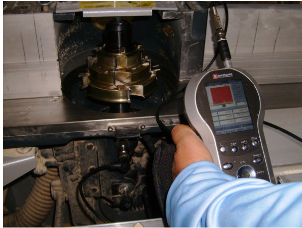
Fig. 2. The connection of the Impaq analyser to milling machinery
