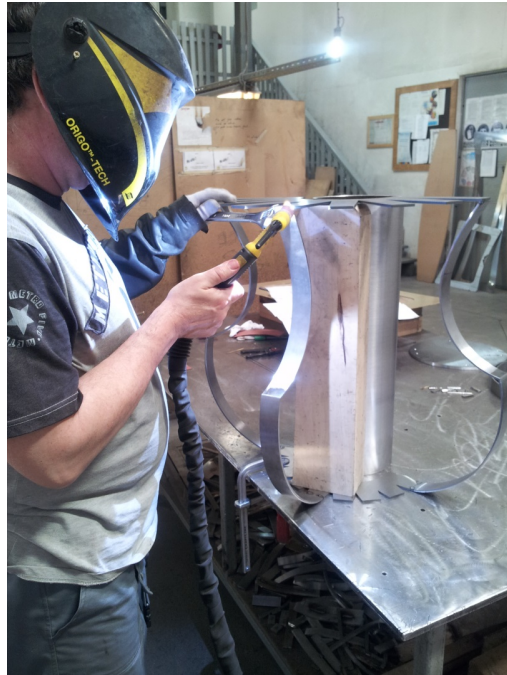
Image 4. Welding steel bands.
