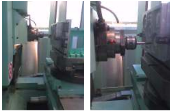
Fig. 2. Stages of the manufacturing of the Al mold by using the processing center
