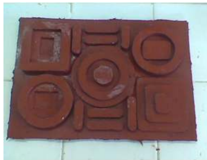
Fig.5. The silicone mold for gypsum casting
