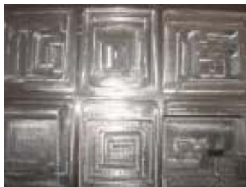
Fig. 3. The Al matrix obtained by machining by using the MC 550PN center
