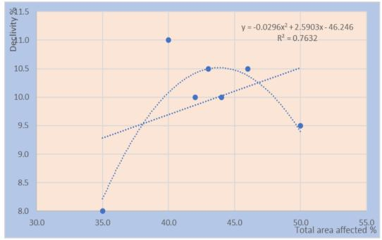
Fig.2. Graphical representation of the polynomial correlation between the declivity and the total affected area resulting on the Arineş forest road
