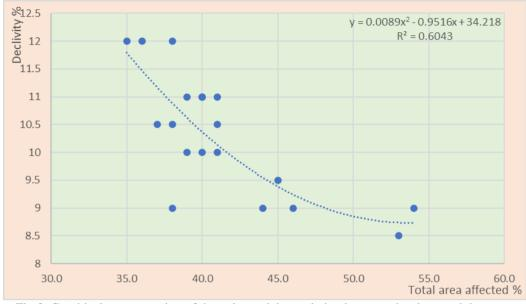
Fig.3. Graphical representation of the polynomial correlation between the slope and the total affected area resulting on the Izvorul Ursului forest road
