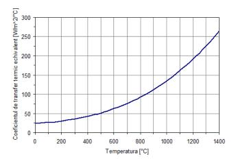
Fig. 4. The temperature dependence of the equivalent heat transfer coefficient in this case
